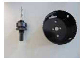
Holesaw, Ø 102 mm, with tool holder for a driller
