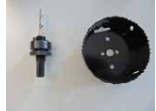
Holesaw, Ø 102 mm, with tool holder for a driller
