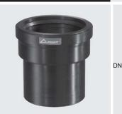
Smooth material transition in domestic range between HD-PE pipes (SDR 33 - SDR 17) and PVC/PP pipes. HD-PE side can be fused with FRIAFIT AM sewage coupler, bends ABM/ABMS or with the outlet of the FRIAFIT ASA-TL sewage saddle. PVC/PP side as socket coupler with SBR lip seal gasket and large insertion depth.
