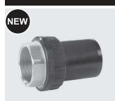
Compact fitting, spigot allows for assembly irrespective of its position and homogenous fusion joint with all suitable FRIALEN fittings. Brass side permanently and tightly connected with PE spigot. Cannot be released or rotated.
