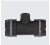
With exposed heating coils for optimal heat transfer, large insertion depth, wide fusion zones plus cold zones at the end and in the middle to prevent the flow of molten material, for use without holding devices. Separate fusion zones. Outlet spigot SDR 11 for processing of UB/MB couplers. Other branch dimensions can be created using MR d 225/160 or MR d 110/90 and MR d 110/63. Handling at the construction site is made easy thanks to the fused-on eyebolts.
