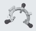
Dimension-bound scraper tool for the reliable removal of the oxide layer of HD-PE and PE-Xa pipe ends and in the saddle area. Scraper blade designed as turning blade with 2 blades (twice the service life). Easy clamping thanks to the open design of the scraper tool.
