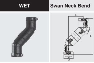
Compact fitting for jointing of pipes which are not aligned and for jointing of service lines with DAA/DAV pressure tapping valves when parallel-installing two mains with identical overlap height. With exposed heating coils for optimal heat transfer, large insertion depth, wide fusion zone plus cold zones at the end and in the transition area to prevent the flow of molten material for use without holding devices.
