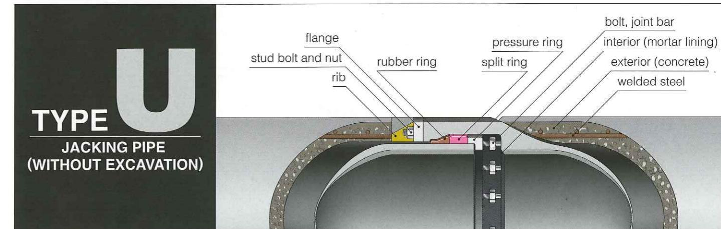
The exterior of T and U type joint pipes (JIS) is wrapped in reinforced concrete, with the exterior diameter of the pipe and joint made to match, smoothed, and the flange and rib welded on the circumference of the spigot have contact with the end surface of the faucet; thus transferring force.
