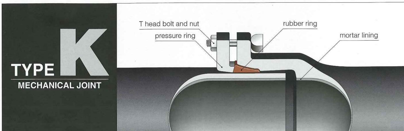
Our standard mechanical joint is extremely water-tight, making it perfect for larger diameter pipes, high-pressure pipes or situations involving high external pressure. The rubber ring, which combines square and rounded rubber components, is bolted through the insert ring, squeezing the rounded portion, and, as in the T-joint, increasing the level of watertightness. It also provides a degree of give as well.
