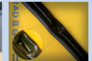
Labelling of a weld bead for traceability reasons
